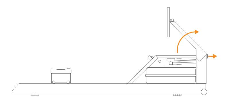
Slide the tablet onto the end of the mounting arm (the speakers should be on the top). Using the tablet bolt and 1/8" Allen key, secure the tablet to the arm.
