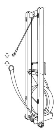
Fill a separate tank with water. Using the siphon, fill the water tank with water to the level 17 marker on the side of the tank. Add a purification tablet (provided in your Ergatta bag).
