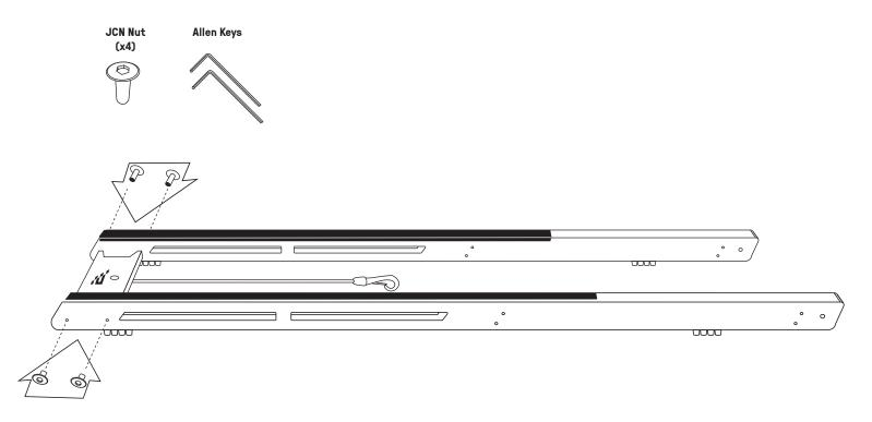
Place the seat assembly between the rails. The indent on the seat should face the rear spacer. Note: it may be necessary to separate the rails slightly to fit.
