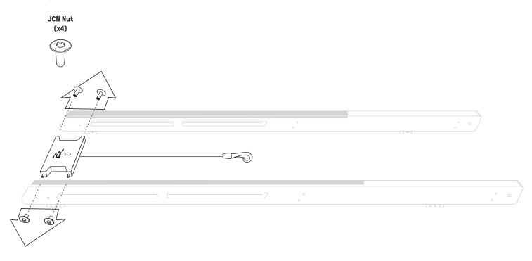
Connect the rear spacer to the rails.
