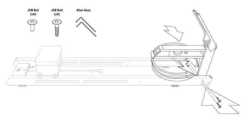
Place the tank assembly between the rails. Using the JCN nuts and JCB bolts, attach the tank to the rails. Use the 5mm Allen keys to screw and tighten.
