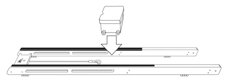
Unscrew the wheel assembly and attach the wheels to the outside of the rails. Screw in the wheels using your hands, then use the 5mm Allen key to tighten.
