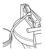
Raise the mounting arm, gently pull the spring lock on the back of the forward riser, and raise the arm until it locks in place.
